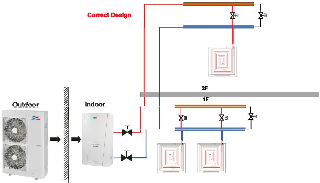
5) Distance between the unit and the water trap (collector) should be within 15m. If the distance exceeds 20m, then it is required to calculate the hydraulic power.
