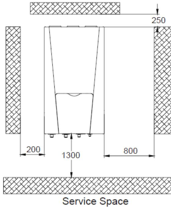
(1) Indoor unit shall be vertically mounted on the wall of the room with expansion bolt.
