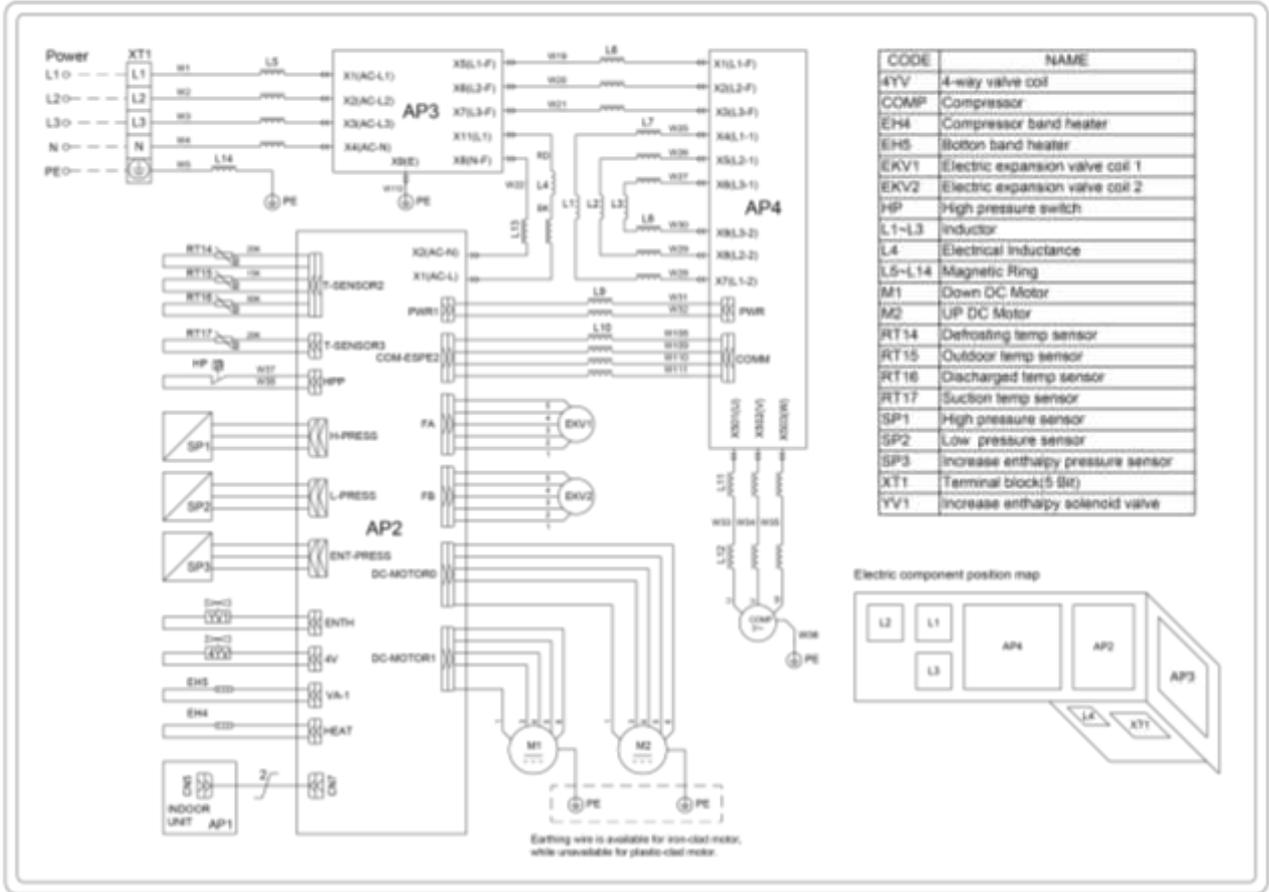
Earthing wire is available for iron-clad motor, while unavailable for plastic-clad motor.
