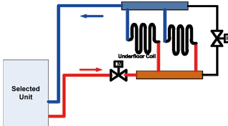
Length of underfloor coils is recommended to be within 100m and length of each branch should be kept the same to the most extent.
