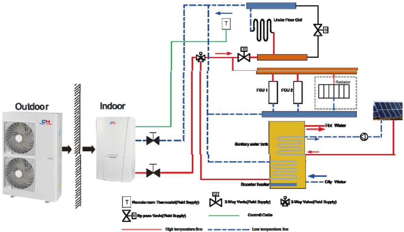
Two-way valve is very important to prevent dew condensation on the floor and radiator while cooling mode.
