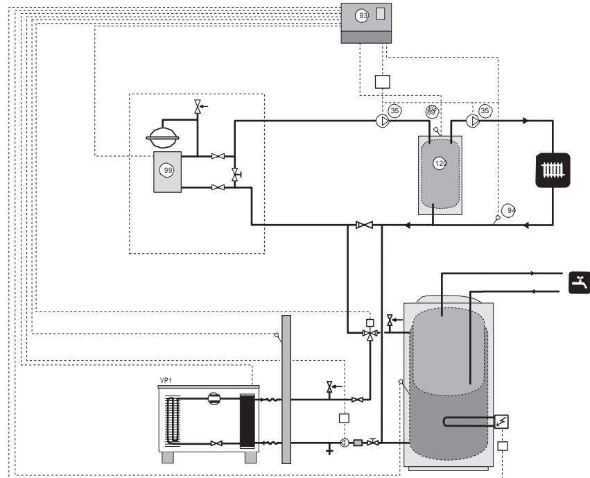
In cases where the system volume in the radiator circuit is below 20 l/kW (heat pump output at 7/45 °C) and/or the radiator flow is choked uncontrolled, a UKV tank is installed as a volume and flow increaser. The T-coupling must be positioned as close to the UKV tank as possible.
