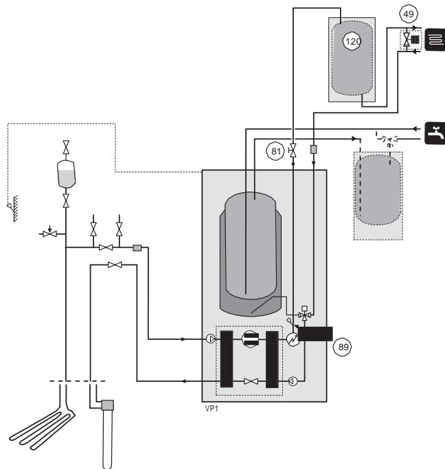
This docking is used when the system volume is insufficient or to reduce heat spikes in the heating system. To eliminate heat spikes in the heating system, a UKV tank is installed. Select diagonal connections (e.g. left up and right down). Plug any connections that are not used. An automatic by-pass valve must be installed if there is a risk of potential 0-flow.
