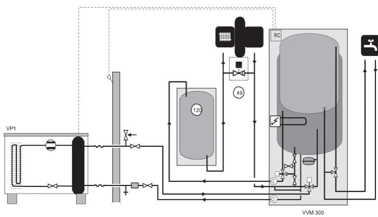
In cases where the system volume in the heating system is below 20 l/kW (heat pump output at 7/45°C) and/or the flow is choked uncontrollably, a UKV tank (120) is installed as a volume and flow increaser. Plug any connections that are not used. An automatic by-pass valve must be installed if there is a risk of potential 0-flow.
