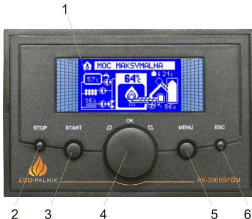
Figure 1. Face plate of RK-2006SPGM governor.
